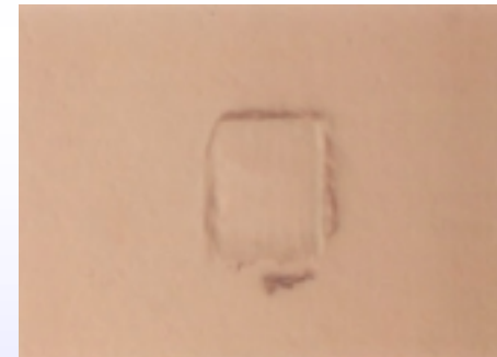
Scrub mark size; 10 \mu\text{m} \times 15 \mu\text{m}
