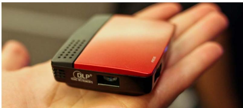
Figure MEMS9 *TI's prototype USB picoprojectorHD Pico with 20 lumens, 640 x 360 resolution, a contrast ratio greater than 1,000:1, a true RGB LED wide color gamut and reliance on a low-power Pico DPP2601 2607 ASIC processor.*
