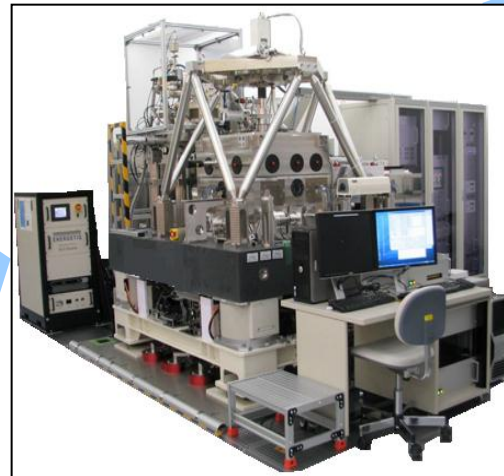
Proto by MIRAI-Seleto (2006-2010) full mask area ABI inspection
