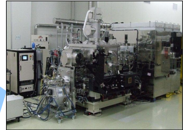
HVM by EIDEC (2011-2015) ABI for hp16nm HVM w/ Lasertec
