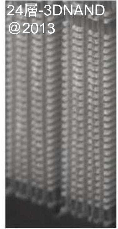
ISSCC2014, Three-Dimensional 128Gb MLC Vertical NAND Flash-Memory with 24-WL Stacked Layers and 50MB/s High-Speed Programming, Ki-Tae Park et al.
